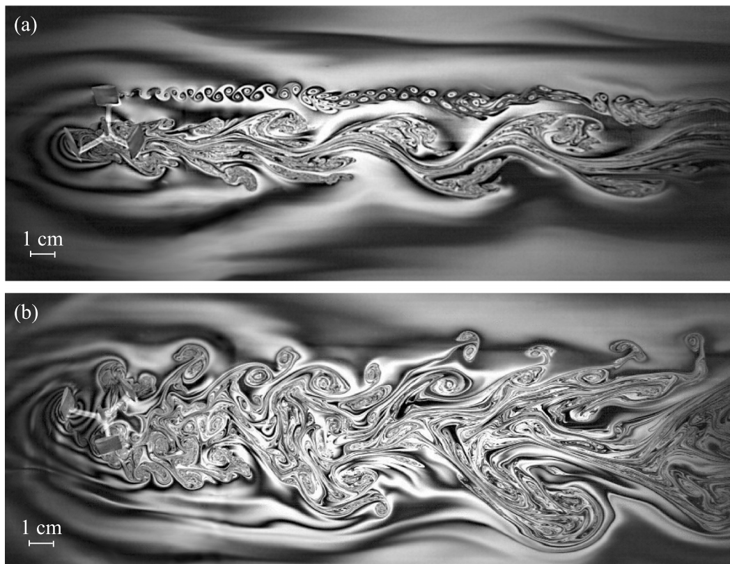
FIG. 1. Soap film visualization of a (a) stationary and (b) clockwise rotating vertical axis wind turbine (VAWT). The incoming flow was gravity-driven and the turbine rotation was motor-driven. The Reynolds number was Re \approx 3000 in both cases, based on the chord length ( L = 0.01 m) and estimates of freestream velocity ( U \approx 2.2 \text{ms}^{-1} ) and kinematic viscosity ( \nu \approx 7 \times 10^{-6} \text{m}^2 \text{s}^{-1} ). The tip speed ratio (blade speed/freestream speed) in the rotating case was TSR \approx 1.04 . The interference pattern created by a monochromatic light source (sodium lamp) convects with the flow and illustrates the intricate structure of the spatially evolving wake. Most striking is the range of scales present in the wake. This is clearly visible not only in the stationary case but also apparent in the rotating case, with small-scale vortices shed from the blades in the near wake and large-scale vortical structures that develop in the far wake. Source: APS-DFD ( http://dx.doi.org/10.1103/APS.DFD.2014.GFM.P0007 ).
