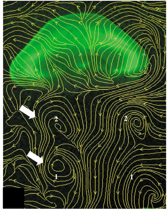
Fig. 9. DPIV measurements of a free-swimming Aurelia aurita jellyfish. Images are taken in the laser sheet plane, which is aligned close to the plane of symmetry of the animal. Vortex wake of the free-swimming jellyfish consists of a train of nearly axisymmetric vortex rings (white arrows; cores numbered in order of formation). Flow field is approximately 14 cm in height.
