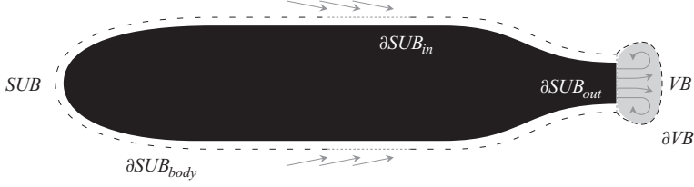
FIGURE 3. Combined vehicle–wake control volume. Vehicle is indicated by black silhouette and wake vortex is indicated by grey patch. Dashed and dotted lines indicate the boundary of combined control volume. See text for symbol definitions.
