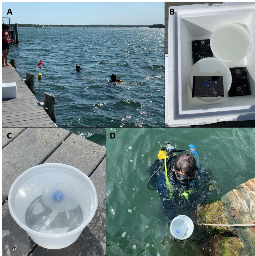
Figure 6. Field experiments conducted in coastal conditions in Woods Hole, MA. A. Swimming experiments in the coastal waters of MA required two SCUBA divers and one person on shore. The person on shore can tie the rope to the dock post and maneuver the biohybrid robotic jellyfish to one diver (illustrated in D), who can release the jellyfish at the bottom of the ocean near the rope as a background feature. The second diver can record videos of the
